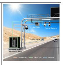
powered devices (PDs) and performed configuration and connection with just a few clicks. It was also used for failure checks and auto reboots to ensure that all the connected cameras and illuminators were working properly. If a reboot of a PD couldn?t solve the problem, engineers could now check on the problem through the web console or viewing the PoE link status shown by the LED indicators on the switch?s front panel.
